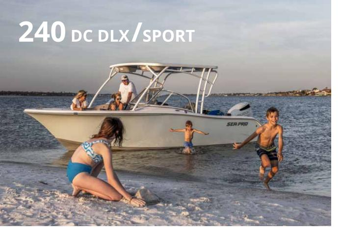
Length 23' 9" Beam 8' 10" Fuel 102 gal. Max HP 350 Livewell 30 gal. Fresh Water 20 gal. Deadrise at Transom 18.5° Draft 16" Bow Fish Box 130 gt. Fish Box Floor (optional) 180 qt. Cooler Box 90 qt. Passenger Capacity 10
