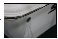
NOTE: The bilge pump is wired to have a constant power supply from the batteries, even when the Battery Selector Switch is turned to the "OFF" position. This allows the bilge pump to operate when the vessel is left unattended. It is important to keep debris and build up away from the Free-Float switch to prevent unnecessary pump operation and drain of the batteries.
