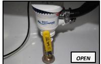
Fully insert the overflow drain pipe. This ensures the livewell will hold water and will not befilled beyond the maximum intended level.
