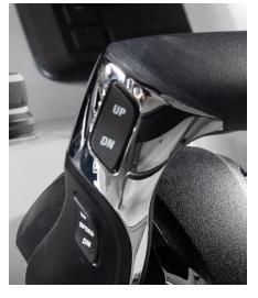
Trimming the motor "down" refers to bringing it closer to the transom. Trimming the motor "up" refers to moving it further away. Utilize the Trim to adjust the angle the vessel will run in the water to optimize performance. *Tilt* refers to the position of the motor
