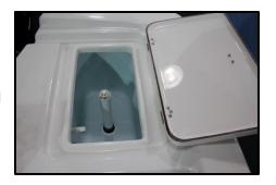
To drain your Livewell, flip the switch on the Helm Switch panel to turn the pump off, close the seacock, and remove the overflow drain pipe.
