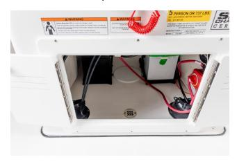
This switch allows the operator to provide power to and disconnect power from the operating systems.
