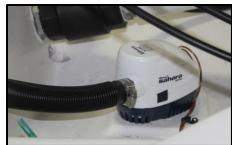
The bilge pump can be manually operated with the switch located on the Helm Switch Panel labeled "PUMPS - BILGE", and is also automatically activated by a Free-Float switch that turns the pump on when water collects inside of the bilge to a predetermined level. This allows the pump to perform it's operation when the vessel is left unattended.
